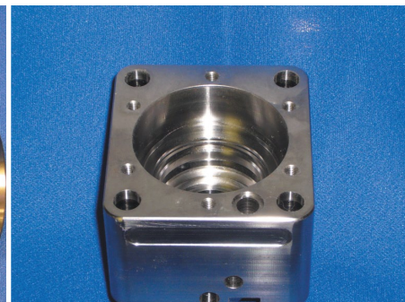
Left photo: ER Collet Spindle for OD Holder on Mori Seiki NLX Series. Right photo: Housing for OD Holder on Mori Seiki NZX Series.
