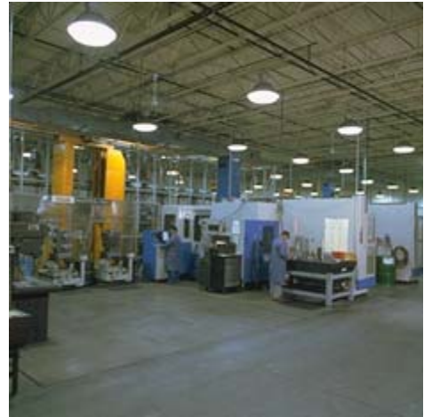
The Mazak Mazatrol Flexible Machining System (FMS). The FMS cell features three horizontal mill machining centers, each served with a 120 tool capacity automatic tool changer. A vertical pallet staker crane robot delivers pallets to the machining centers. Set-up time is reduced to zero. Raw casting to finished, inspected parts all completed within the FMS cell, making very short lead times possible.
