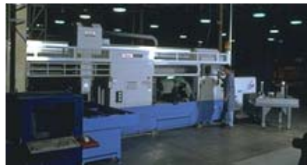
The Multiplex cell features two CNC lathes. Each lathe utilizes dual horizontally opposed spindles allowing for first and second-process machining simultaneously. Option equipment being utilized includes external bar feeder and gantry robot loading. The dual spindles provide the quality required in manufacturing hydraulic and power transmission components while increasing machine throughput and reducing the costs of manufacture.
